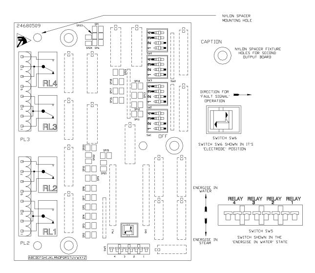
Figure 3b.1 - View of relay output board showing switch positions and output pin details
